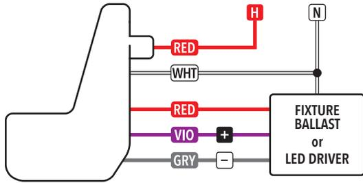
LINE VOLTAGE INTERCHANGEABLE LENS FIXTURE MOUNT: DUAL POLE SWITCHING 2-PHASE (480 VAC)
