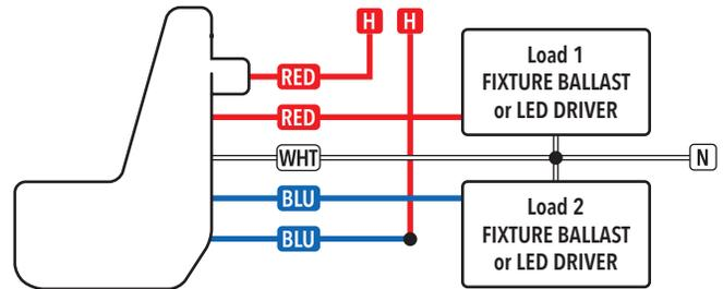
LINE VOLTAGE INTERCHANGEABLE LENS FIXTURE MOUNT: 2-PHASE (MVOLT)
