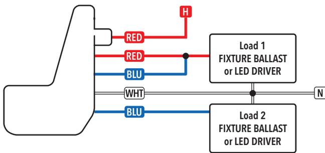
LINE VOLTAGE INTERCHANGEABLE LENS FIXTURE MOUNT: 2-POLE (HVOLT)
