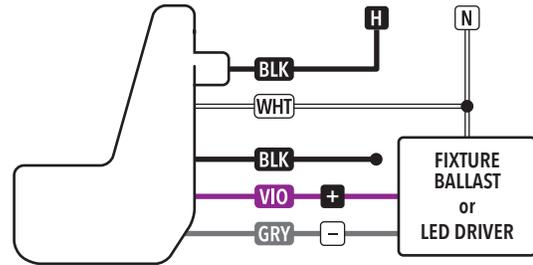
LINE VOLTAGE INTERCHANGEABLE LENS FIXTURE MOUNT:
