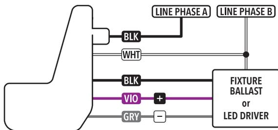
LINE VOLTAGE INTERCHANGEABLE LENS FIXTURE MOUNT: 2-PHASE (HVOLT)
