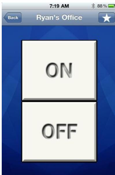
Notice that the switch is backlit, indicating that the **relay** controlled by this nLight Virtual WallPod is **closed**, i.e., “turned on.”
