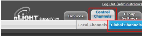
To create groups of devices that will switch on and off together, click on the Control Channels tab at the top right of the page followed by the Global Channels tab. The tree will expand and display all of the devices that can broadcast and track events over the nWiFi network.
