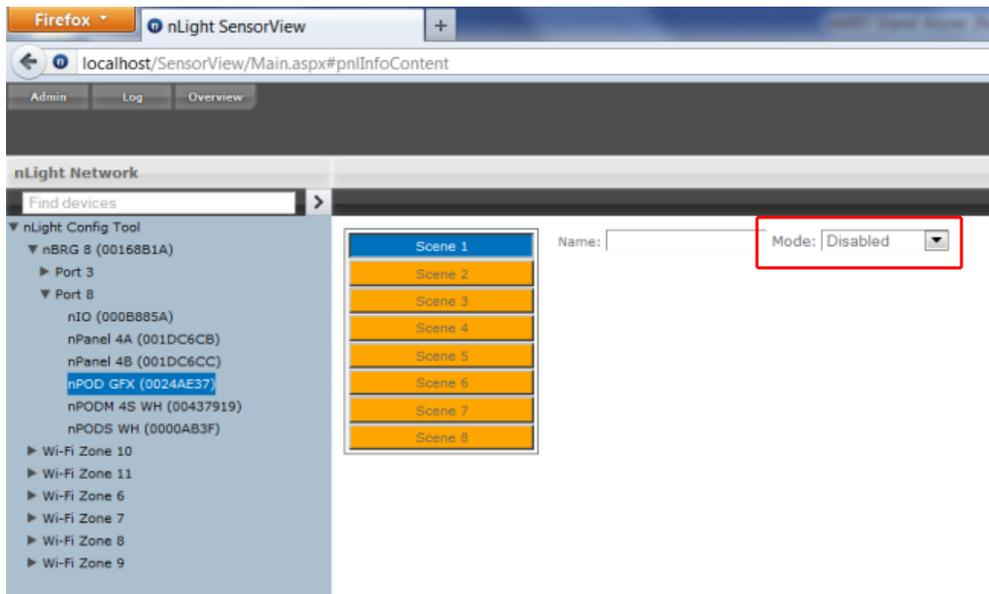
Change the mode to Global Preset **Mode:**  and select the desired global channels. Once they have been selected set them to On, Off, or a Dim Level (if dimming hardware is installed) and click Save.
