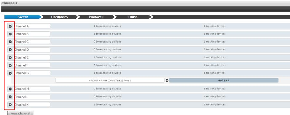
Any Global Channels that have been previously assigned will be displayed. A maximum of 128 Global Channels are available. To view or edit the devices that are part of a global channel expand the channel by clicking the arrow next to the channel name. Click the box under Broadcasting Devices or Tracking Devices to add or remove devices from that group using the device tree.
