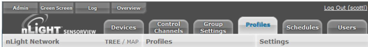
The **Profiles** tab is where control modes and settings for a particular group are selected. A schedule (complete with a recurrence pattern) and priority are also chosen on this page.
