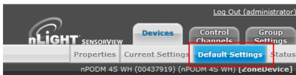
To set a Global Preset for an nPOD(M) device, find device in the tree on the Devices page and select the Default Settings tab near the top right of the page.
