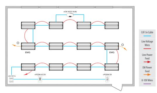
Note: Not all emergency nLight enabled fixtures require a normal monitoring feed. Refer to data sheet for additional information.
