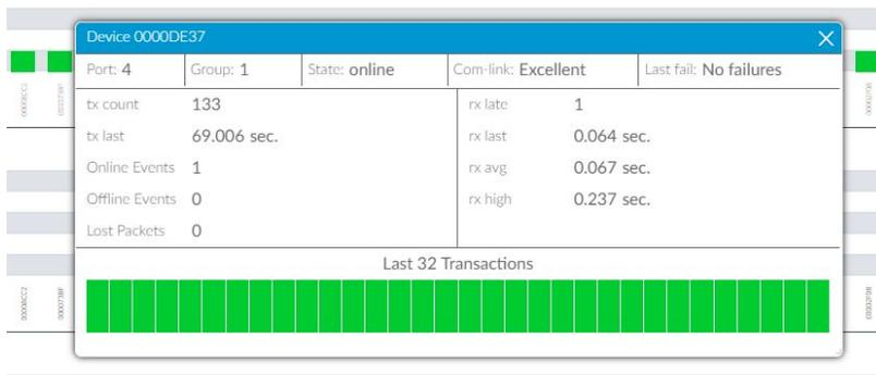
Selecting any individual nLight Air device will bring up a window with additional debugging data for that device. In addition to running counts of successful and unsuccessful transactions and time statistics for transaction times, there is a graphical display of the most recent transactions (green for successful transactions, red for unsuccessful transactions). Up to 32 transaction results can be displayed (less if there are fewer transactions to that particular device).
