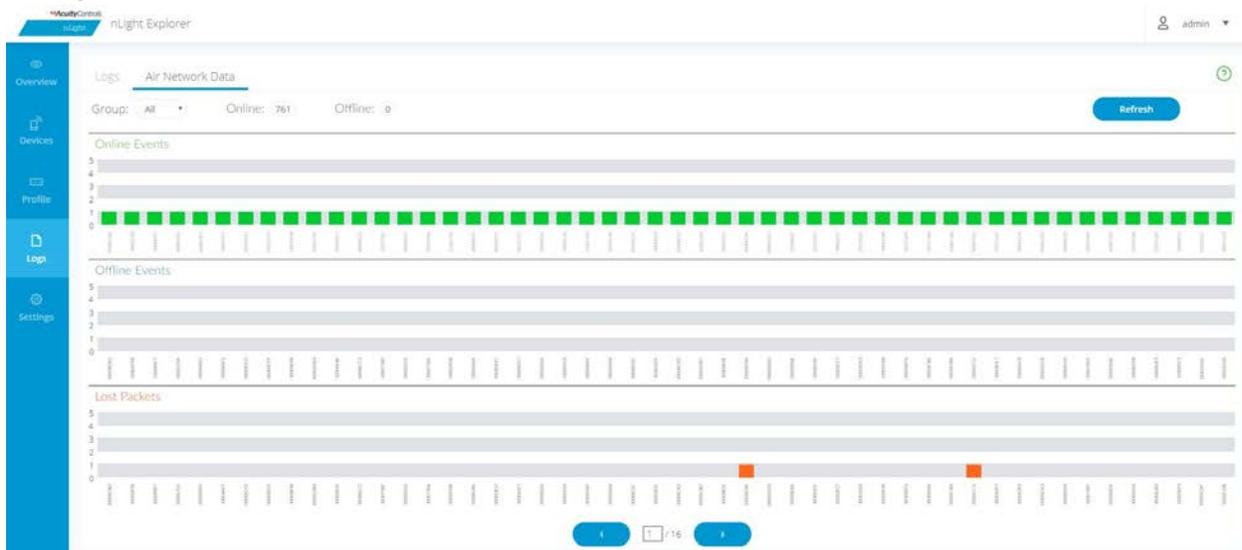
For nLight systems that include nLight Air wireless devices, the "Air Network Data" section provides additional analytics regarding the communication stability between the nLight ECLYPSE and nLight Air devices. Selecting this option provides the following:
