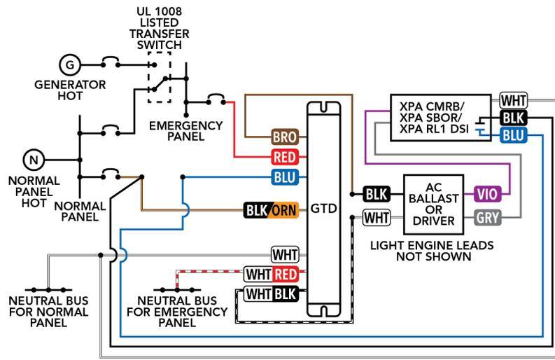
Figure 6: Example Wiring Diagram - GTD with XPoint Wireless Controller
