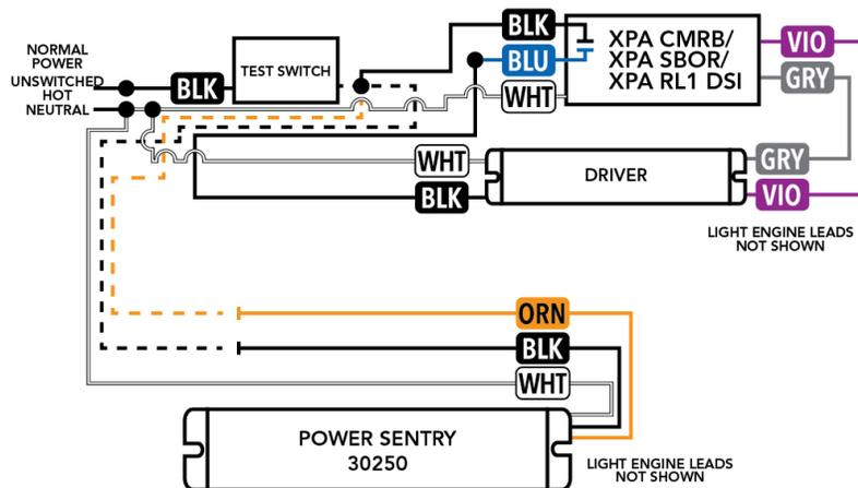
Figure 4: Example Wiring Diagram - Power Sentry PS30250 battery powered emergency driver with XPoint Wireless Controller
