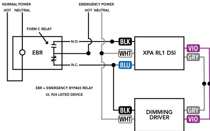
Figure 8: Example Wiring Diagram - Emergency Bypass Relay (Form C) with XPoint Wireless Controller
