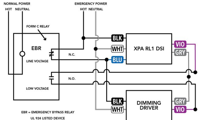
Figure 9: Example Wiring Diagram - Emergency Bypass Relay (0-10V Interrupt) with XPoint Wireless Controller
