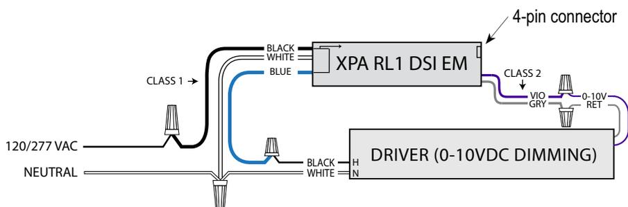
Figure 2 - Example EM Wiring Diagram: XPA RL1 DSI EM
