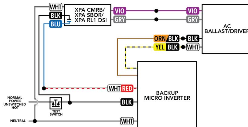
Figure 7: Example Wiring Diagram - Backup Micro Inverter with XPoint Wireless Controller
