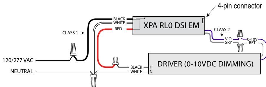
Figure 3 - Example EM Wiring Diagram: XPA RLO DSI EM
