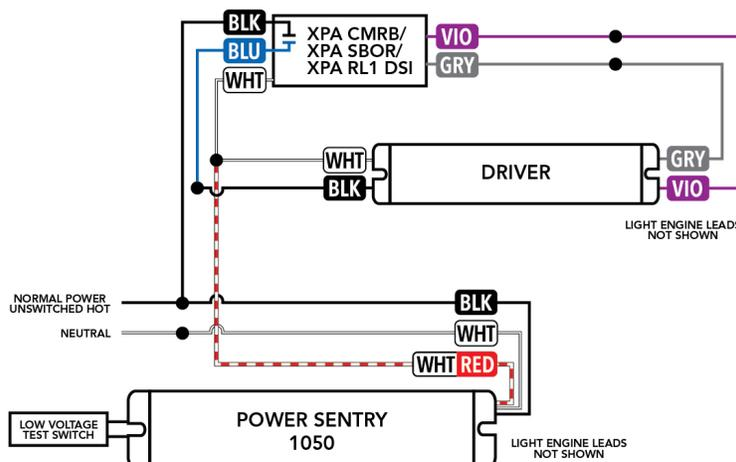
Figure 5: Example Wiring Diagram - Power Sentry PS1050 battery powered emergency driver with XPoint Wireless Controller
