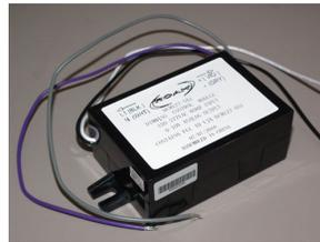
**MacID** - The 8 digit hexadecimal MacID is ROAM's unique identifier assigned to the internal radio of all nodes and DCMs. The values of the barcode MacID will only consist of hexadecimal values, 0-9 or A-F. Once activated, this MacID is associated with the light on which it is mounted. All attributes and location captured at installation create a one-to-one association between the light and the ROAM node, which is why it is important to follow ROAM node replacement processes.
