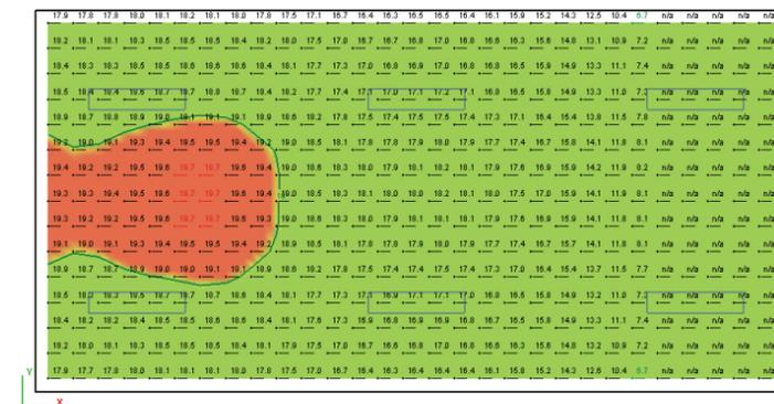
Figure 2. A typical UGR calculation result, for an observer looking east.
