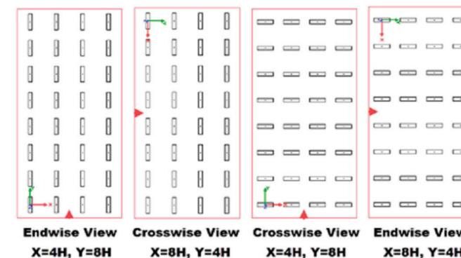
Figure 1. Examples of the four standard observer positions used in UGR calculations.
