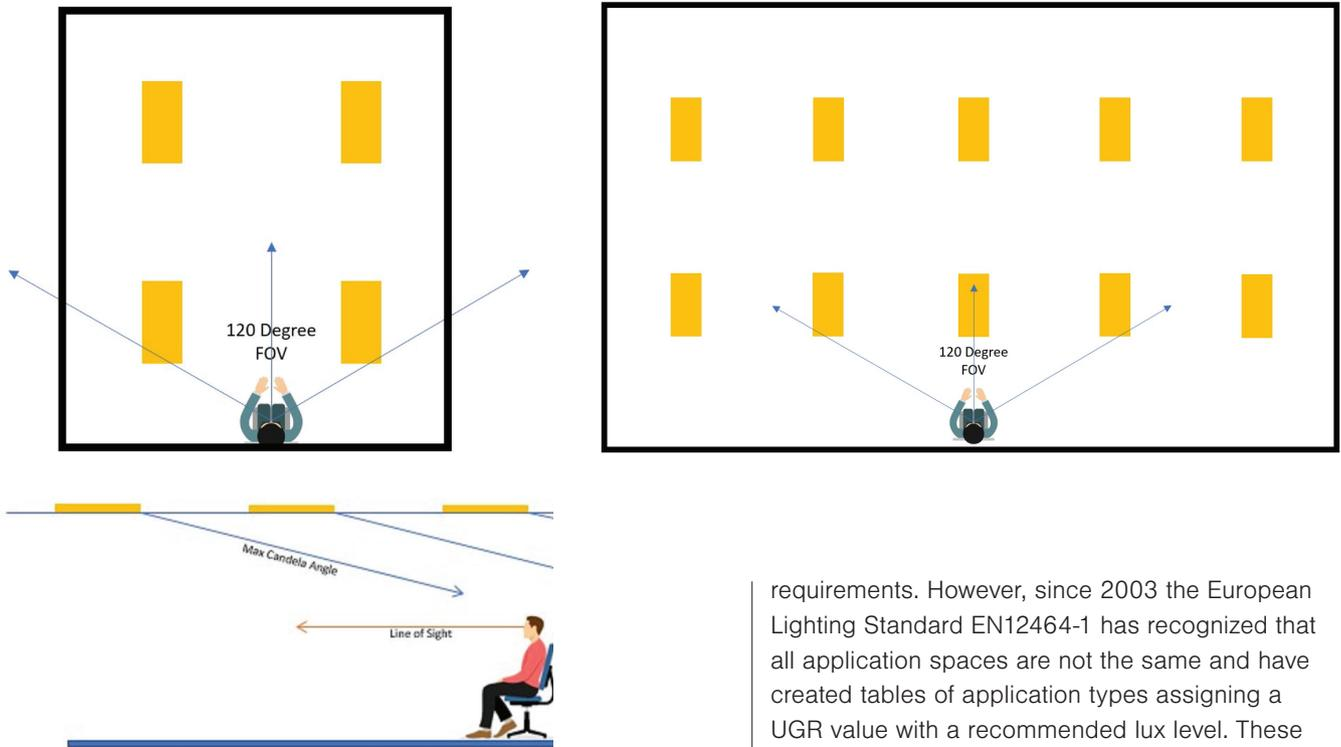
Figure 3. An example of luminaire max-candela angle shown with respect to observer line of sight.
