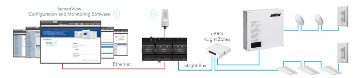
Whether triggered by a schedule, a photosensor, wall station or occupancy sensors, the nLight Relay Panel automates energy savings and supports commercial building energy code compliance by delivering scheduling, daylight, dimming, and occupancy control.
