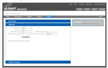
This interface is a BACnet/IP software solution that requires the SensorView application to run at all times. The SensorView host server must be permantently connected to the network of nLight hardware devices. BACnet is not resident on nLight hardware devices, SensorView manages all BACnet communication on behalf of the hardware. The following requests for nLight network and device information are supported:
