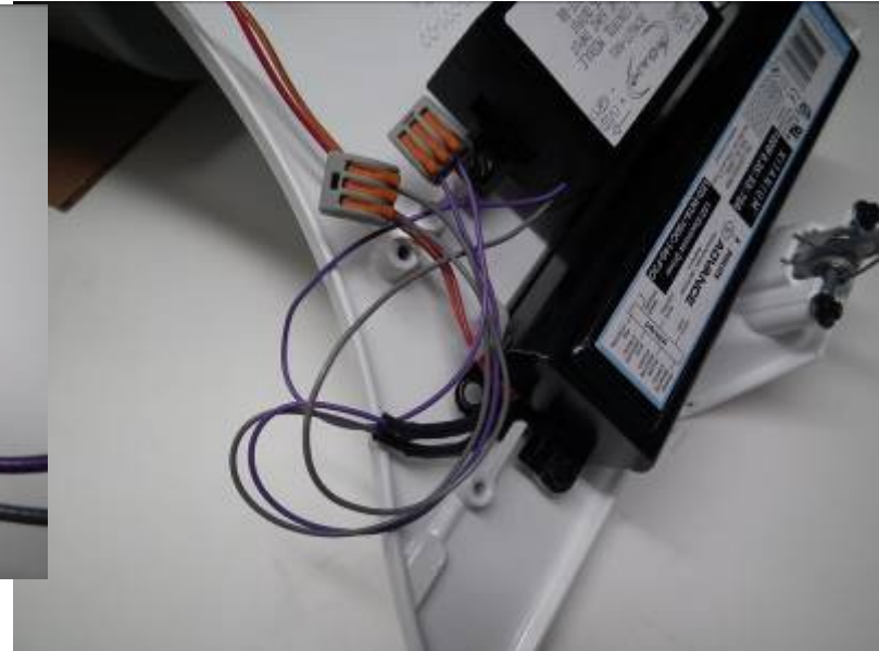
DCM VIOLET AND GREY WIRES CONNECTED TO DRIVER VIOLET AND GREY WIRES (TOOL-LESS TERMINATION STYLE SHOWN)
