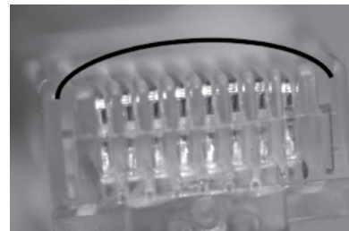
Contacts not seated properly (bowed crimping).
