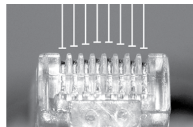
Contacts not seated properly (bowed crimping).
