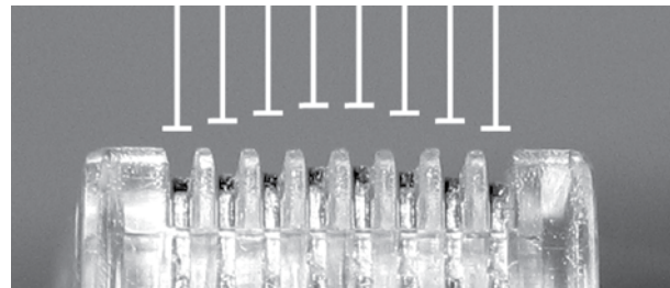
Figure 1.9b: Contacts are not seated properly.
