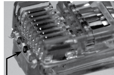
Contacts not seated properly (sticking out 1/16 of an inch too far).
