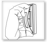
TIP: To remove the trim plate, use a flat-head screwdriver to depress the trim plate tabs using the 2 slots on the bottom
