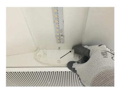
C. Ensure safety glasses and gloves are on. Break both removed Light Traps in half and discard.
